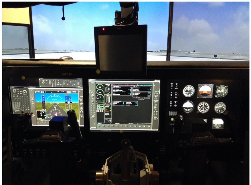
This effort extends ZedaSoft's CBA® for Simulation framework to interface with real aircraft avionics hardware. The CBA framework was previously interfaced successfully to stimulate Cobham IDU-series cockpit hardware on Textron's Scorpion ISR/Strike prototype aircraft development.
