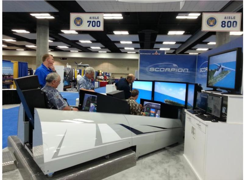
ZedaSoft integrated the simulators with MetaVR's Virtual Reality Scene Generator software to provide the out-the-window visual scene and sensor views to simulate the L-3 WESCAM MX-15 and FLIR Systems EO/IR sensor payloads. MetaVR also developed the aircraft model and delivered it with 50cm satellite imagery for the CONUS, Hawaii and Afghanistan visual scene databases.
